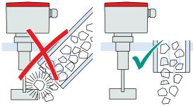
For heavy bulk materials that could damage the shaft or the paddle:
