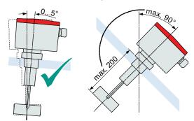
For lateral installation (horizontal shaft): Install the unit in such a way that the cable connections are on the underside of the housing.
